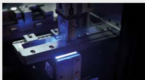
UV Black light provides evidence of eventual traces of hydrocarbons, grease or particulate.
